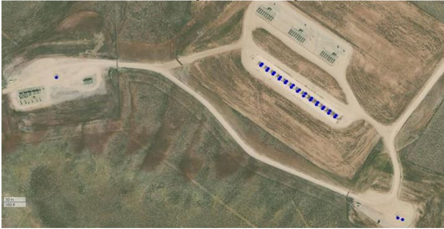
Figure 2-3. Satellite image of three well pads with 1, 2, and 16 wells, respectively, in the Pinedale Field. (Source: Satellite photo from DrillingInfo.)
