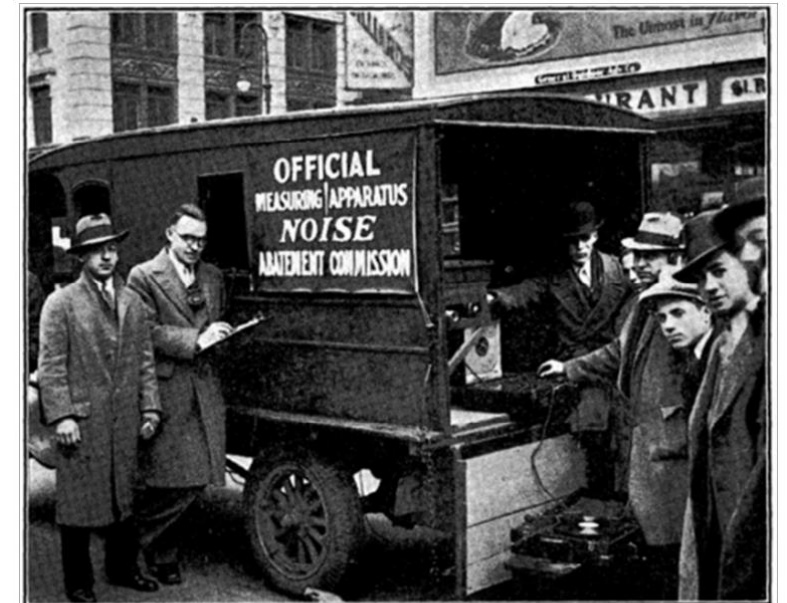
Photograph by Bell Telephone Laboratories The noise measuring truck traveled over 500 miles in city streets, observing noise levels at 138 stations
