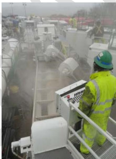
**Figure 14. Generation of silica dust in a hydraulic fracturing operation.** (Source: <http://blogs.cdc.gov/niosh-science-blog/2012/05/23/silica-fracking/>).
