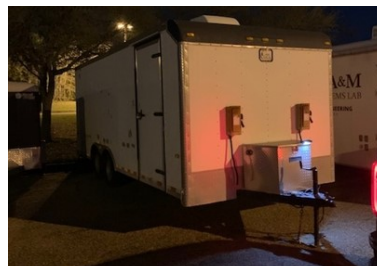
Trailer that is being outfitted with air, radiation, and noise sampling equipment for placement in the Permian Basin and Eagle Ford Shale, Texas.
